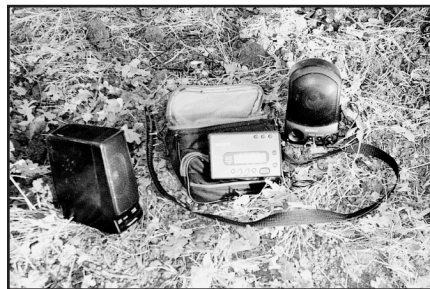
A very compact, lightweight, good-quality playback setup can be constructed from a Sony TCD-D7 or TCD-D8 DAT recorder and a small speaker, both contained within a small padded camera case. Birds can better tell that recorded playback is "fake" if one portion of playback setup is not of top quality. For example, Realistic (Radio Shack) speaker on left has tended to be less effective in attracting warblers than Sony speaker on right.
