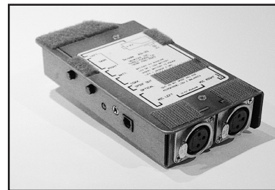
The Denecke AD-20 is a combined microphone preamplifier and analog-to-digital converter offering XLR inputs (no phantom power) and coaxial and optical digital outputs. A proprietary cable is required to use the AD-20 with the Sony D8.
