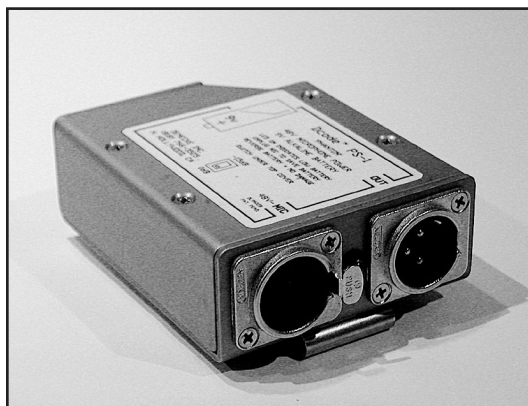
The Denecke Dcode PS-1 provides phantom power to a condenser microphone from a single 9V battery.
