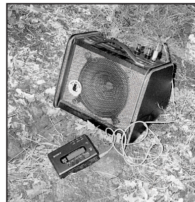
Recorded playback setup using a Sony TCD-D7 DAT recorder and a high quality field-portable speaker (Maxi Mouse, Lectronsonics Corp., Rio Rancho, NM). Assuming one has a good playback machine, effectiveness of playback can vary with quality of playback recording and speaker.
